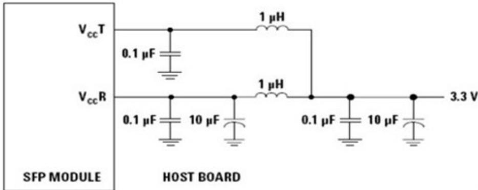
Note: Inductors with DC resistance of less than 1Ω should be used in order to maintain the required voltage at the SFP input pin with 3.3V supply voltage. When the recommended supply filtering network is used, hot plugging of the SFP transceiver module will result in an inrush current of no more than 30 mA greater than the steady state value
