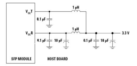
Note: Inductors with DC resistance of less than 1 should be used in order to maintain the required voltage at the SFP input pin with 3.3V supply voltage. When the recommended<sub> $\Omega$ </sub> supply filtering network is used, hot plugging of the SFP transceiver module will result in an inrush current of no more than 30 mA greater than the steady state value
