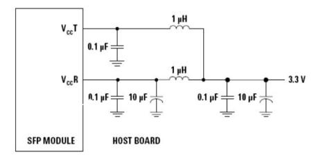
Note: Inductors with DC resistance of less than 1 should be used in order to maintain the required voltage at the SFP input pin with 3.3V supply voltage. When the recommended  $\Omega$  supply filtering network is used, hot plugging of the SFP transceiver module will result in an inrush current of no more than 30 mA greater than the steady state value
